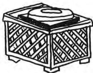
Lattice screen for compressors.
